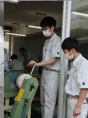
供試体の端面を研磨
